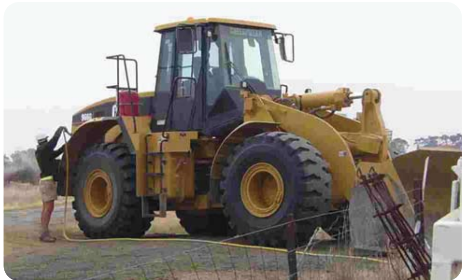
A construction contractor cleans his vehicle as part of the project's weed management strategies
